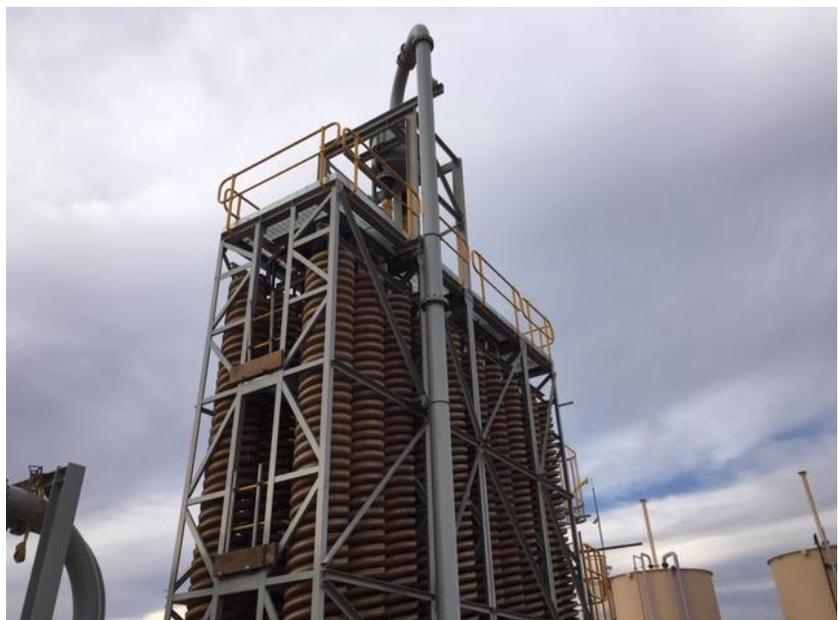
**Figure 4.** Spiral installation
