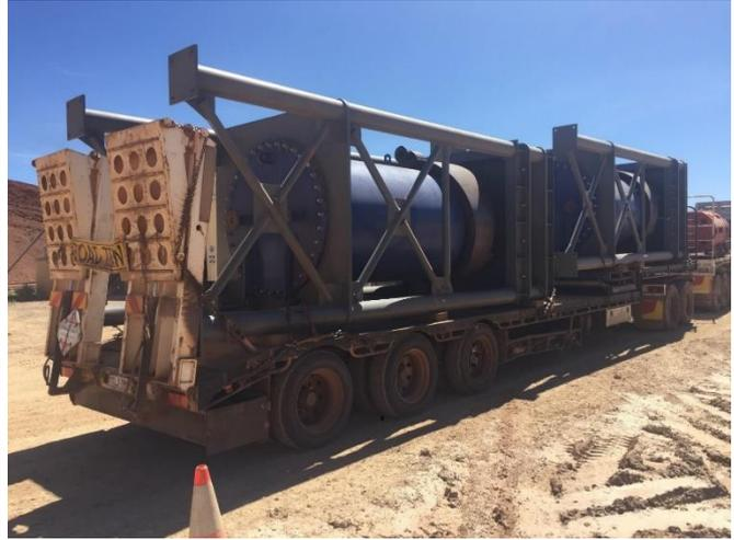
**Figure 6.** Grinding mills arriving on site
